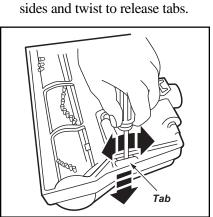
4. Turn Electroglide Powerhead right side up. Press handle release pedal and lower the swivel. Tilt cover forward from back until front snaps free.
